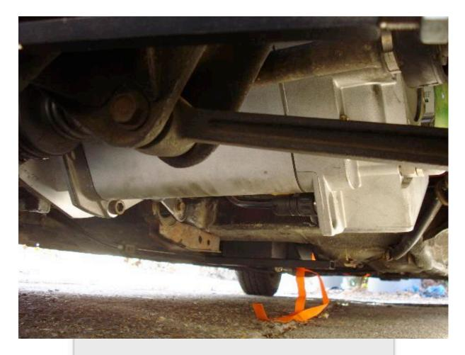
Here you can see how the motor is mounted low in the car but just a little higher than the lowest as defined by the transmission (not shown). The tunnel battery box can be seen just above the orange straps that need to be trimmed.
