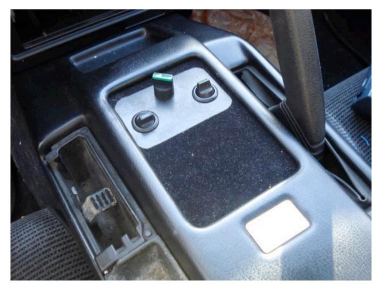
Control panel has drive selector, regen on/off and full power on/off
