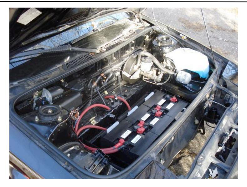
6 modules, the tan cylinder is the brake vacuum reservoir. The vac pump can be seen in the compartment where the radiators used to be
